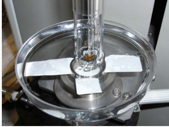
Figure 4.16. Experimental setup of swelling kinetics of HSA plastics using thermomechanical analyzer.
