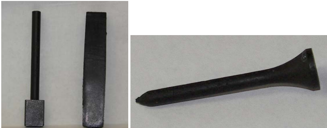
Figure 7.11. Different machined products from the bar of bloodmeal plastics.
