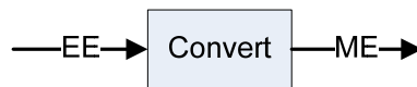
Figure 2.4: Function structure of an electrical motor using the Functional Basis (secondary level)
