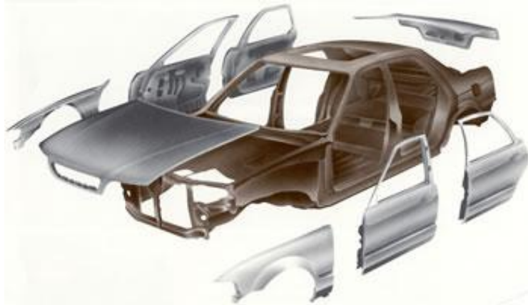
Figure 1.3: Major panels of BIW with closures (AluMATTER, 2011)
