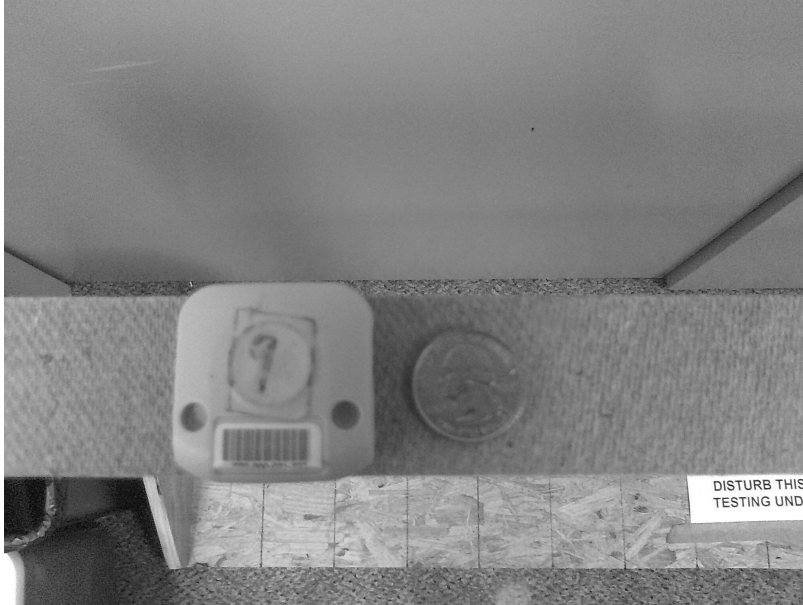
Figure 2.11: Photo of a Ubisense UWB transmitter tag.
