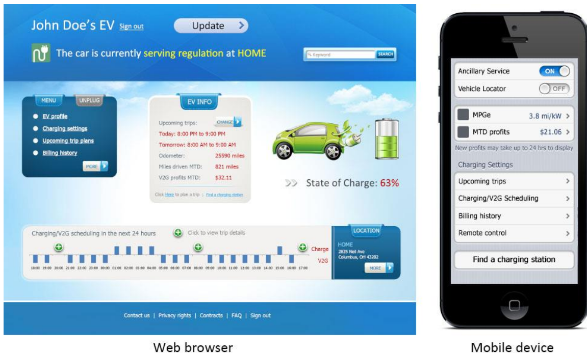
Figure 7. Interfaces of the charging management system on the web browser and mobile device
