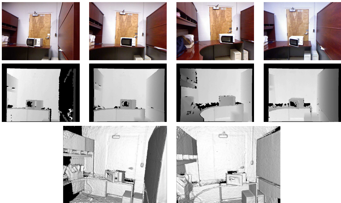
Figure 5.16: Top: Four color images (out of hundreds of recorded) of the microwave in a different configuration. Middle: Four corresponding depth images of the microwave. Bottom: 3D reconstructions.
