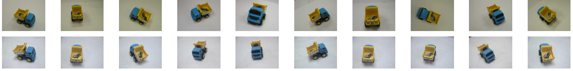
Figure 4.9: Top: Ten images taken at arbitrary viewpoints for pose estimation of the truck. Bottom: The corresponding images that, among all the images used for 3D reconstruction, have the highest number of matched feature points for each image.
