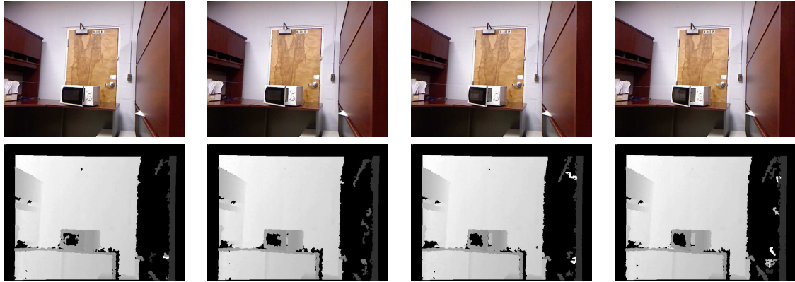
Figure 5.17: Top: Four color images (out of a set of captured) of a microwave as the door is being opened. Bottom: Four corresponding depth images of the microwave.
