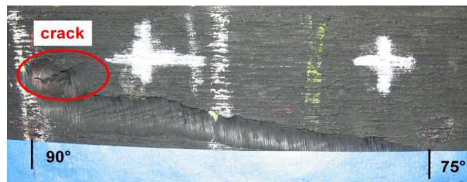
Figure 55: Shearography testing limited by existing surface cracks on a used tire casing
