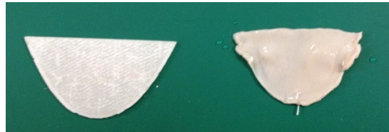
Figure 18: 3D printed cusp mold shown on the left and the pericardium cusp after it had been cut out of the crush mount
