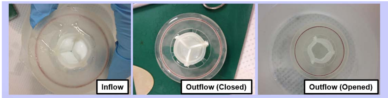
Figure 19: Tissue engineered aortic valve from decellularized and PGG fixed bovine pericardium and sutured into novel mount
