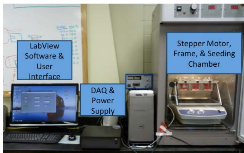
Figure 32: Rotator system consists of the metal frame where the seeding chambers can be secured and is connected to a stepper motor that is controlled by LabView. The system resides in the 37C incubator for cell viability.
