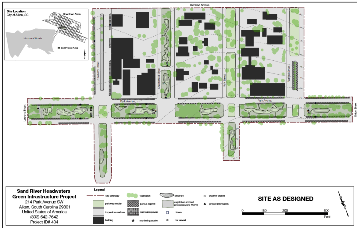
Figure 4-3. Bioretention cell and monitoring locations in downtown Aiken, SC (Sand River Headwaters Green Infrastructure Project, 2010).
