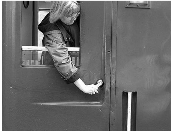
Figure 2.11: A British “slam-door”: an inside user has to first open the window, reach outside, and then turn the exterior handle. Without guideline, this door frustrated many foreigners. (Turner, 2005)
