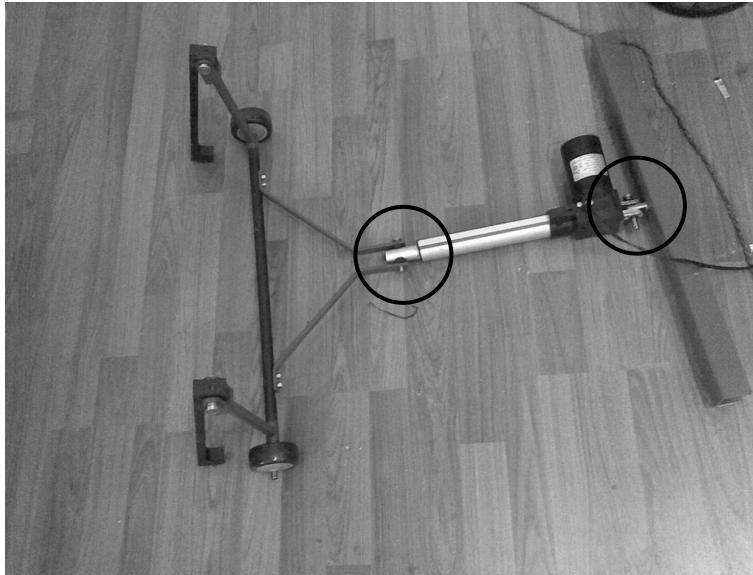
Figure 0.7: The circle-marked joints are manufactured to be connected by pin bolts
