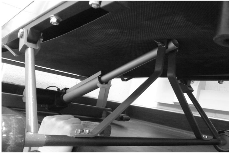
Figure 0.8: The connections by pin bolts afford the unexpected folding of the links
