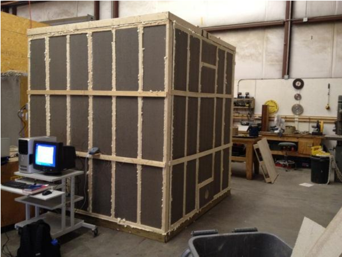
Figure 3-4: The finished experimental room, with the two interchangeable inlet panels shown
