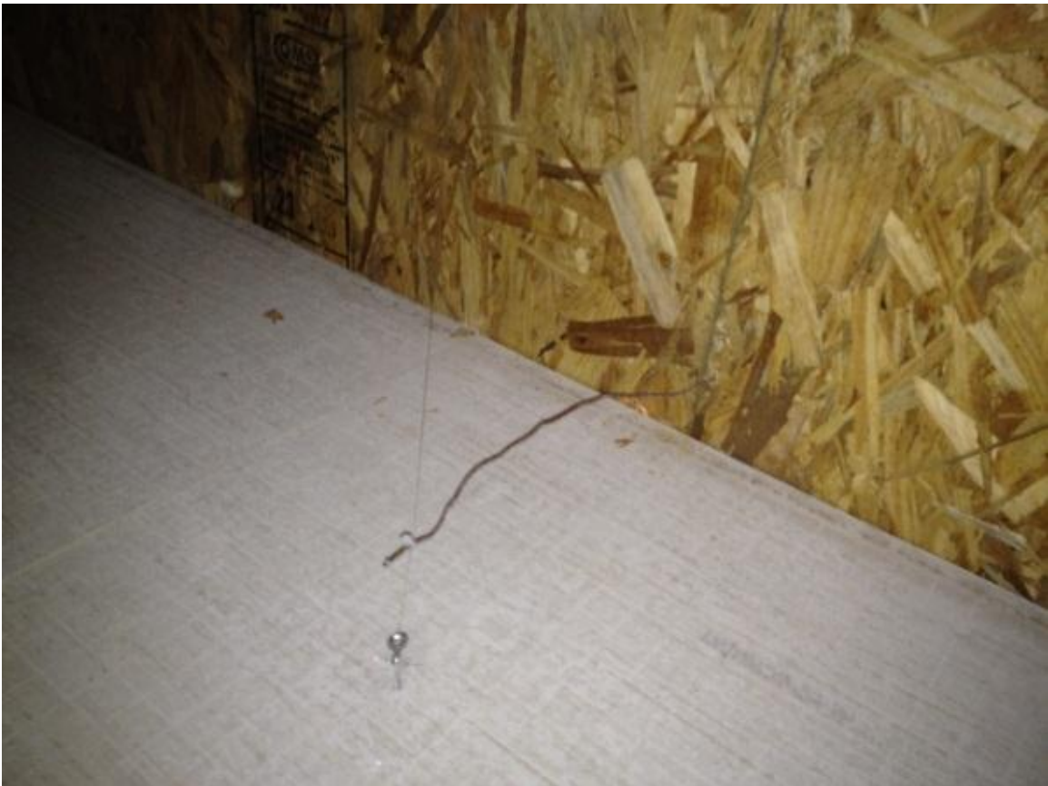
Figure 3-10: The thermocouple closest to the floor of the experimental room
