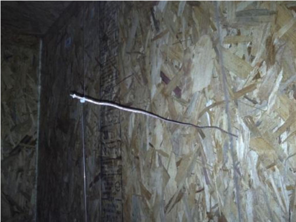
Figure 3-11: A thermocouple inside the experimental room attached to the fishing line with a small zip tie
