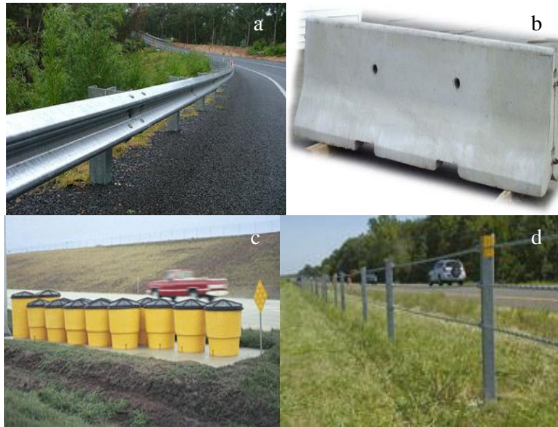
Figure 4.2: Roadway barriers in the United States: (a) guard rail (TLJE, 2012), (b) Jersey barrier (ACI, 2012), (c) Fitch barrier (Enterprise Flasher, 2012), and (d) cable guard (MDOT, 2012)
