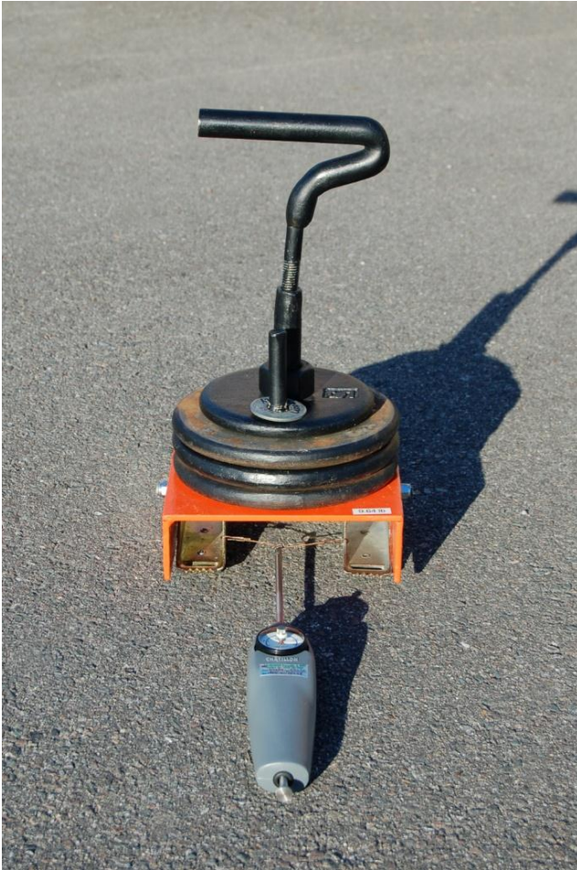
Figure 2.8. The ladder shoes and frame were modified to create a horizontal dynamometer pull-meter for coefficient of friction testing on a variety of surfaces. This procedure is in general accordance with ASTM C-1028.
