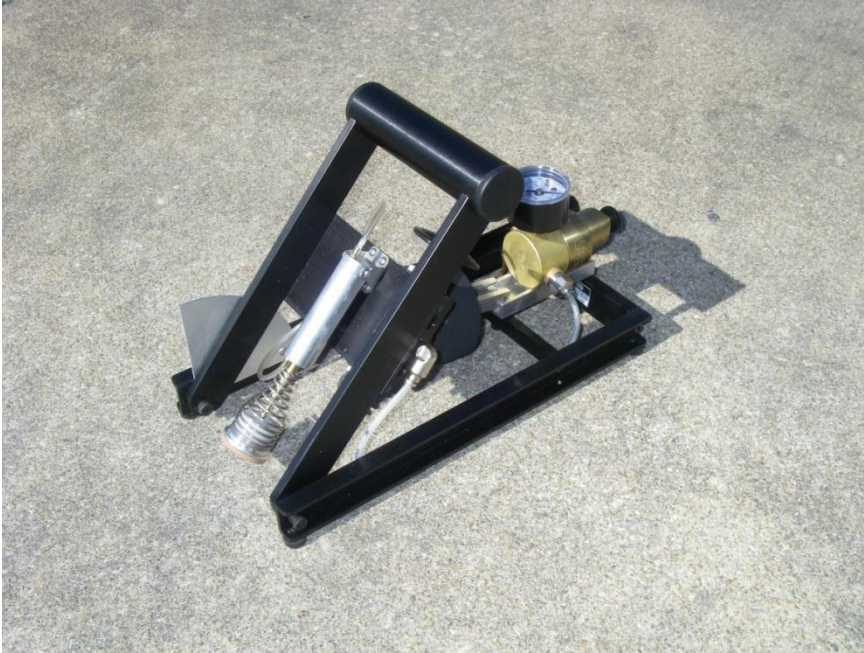
Figure 2.9. Variable incidence tribometer (VIT) for additional coefficient of friction testing.
