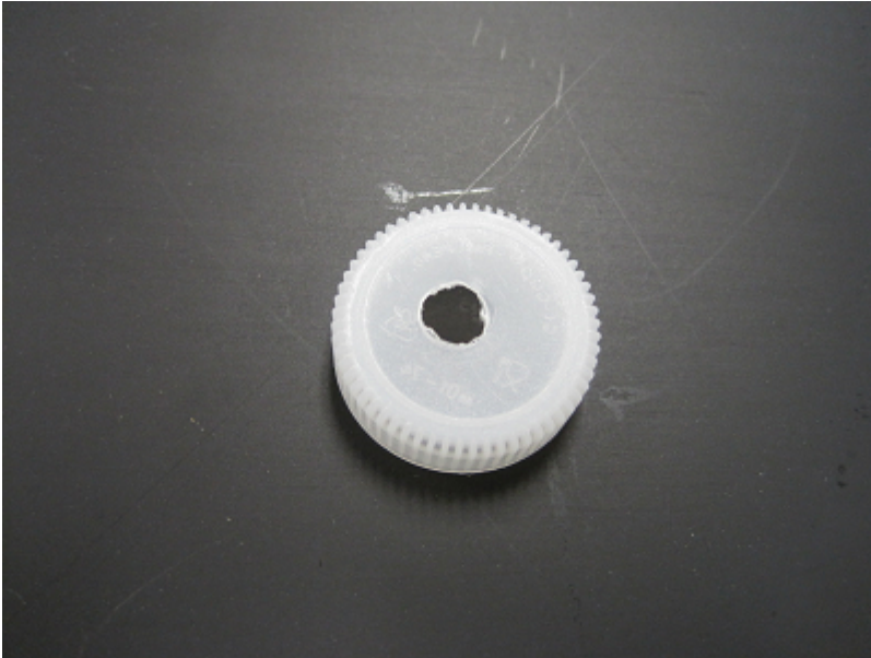
Figure 27. Small Bottle Cap with 0.25in Diameter Hole
