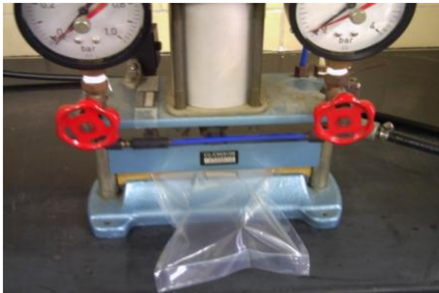
Figure 15. Open Pouch Inflation Burst Tester.
