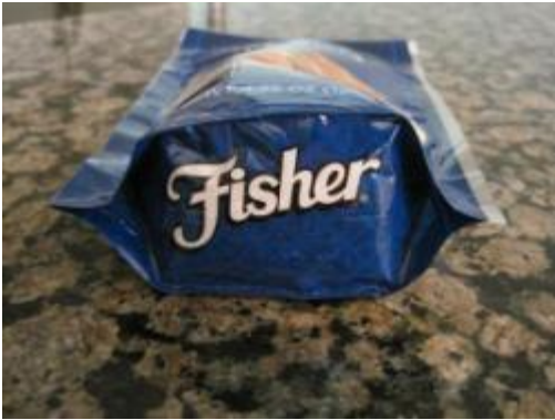
Figure 3. Bottom Gusset on Stand-up Pouch.
