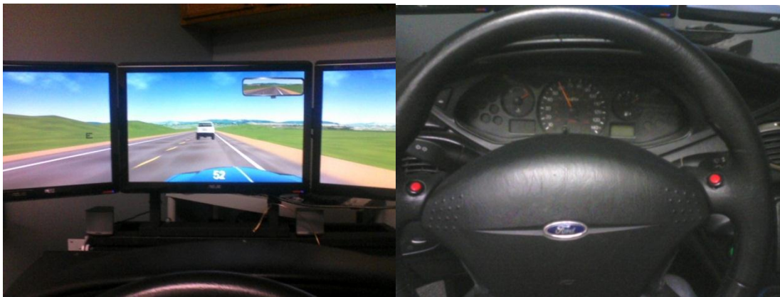
Figure 5(a) (left): Virtual environment with target “E” on the screen. (b) (right) Steering wheel and red functional object detection buttons.
