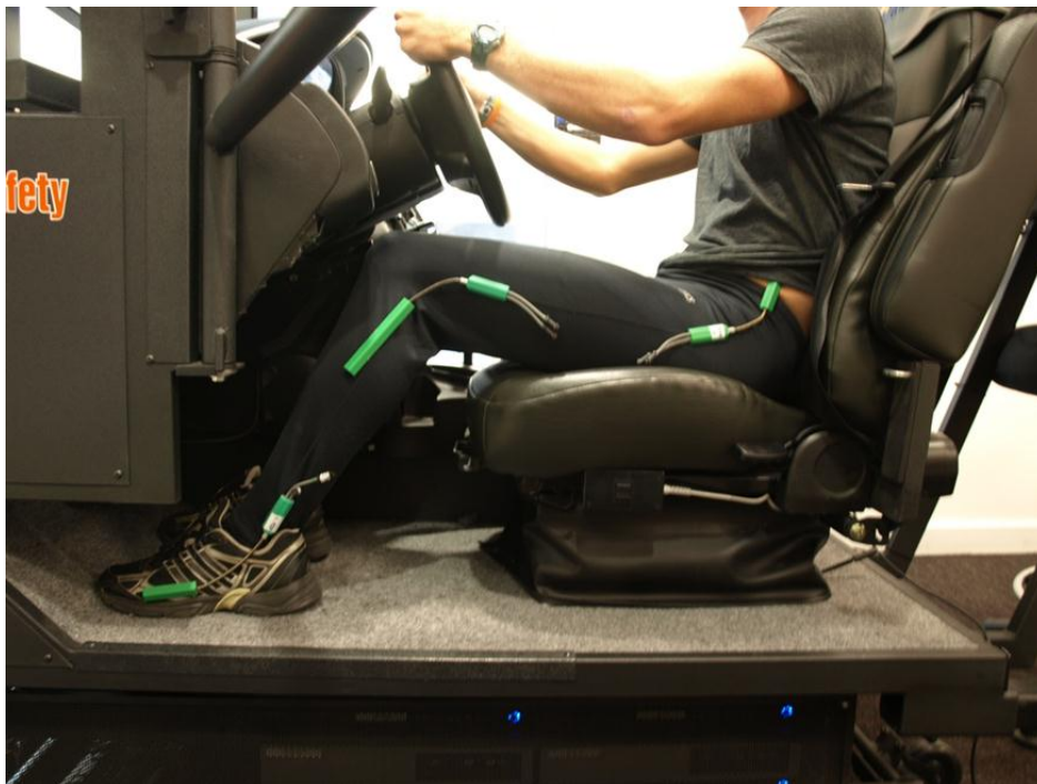
Figure 3: Biometrics placement using a different attachment technique- double-sided medical grade tape.
