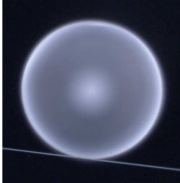
Figure 2.4.2: Micro sphere resonator fabricated by CO 2 laser.
