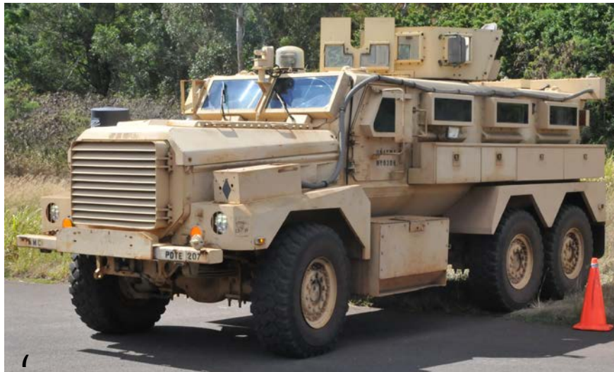
Figure 4–1 Typical light tactical vehicles currently used by the US military: (a) High Mobility Multipurpose Wheeled Vehicle (HMMWV) [3]; and (b) Mine Resistant Ambush Protected (MRAP) vehicle [6].
