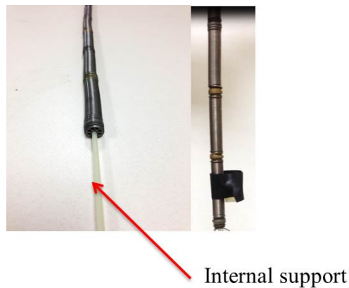
Figure 3.8: Internal support to prevent torsion
