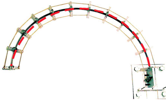
Figure 1.1: Continuum robot with constant curvature segments [1]
