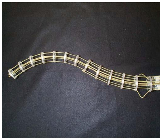
Figure 2.1: Tentacle robot with incompressible flexible backbone rod
