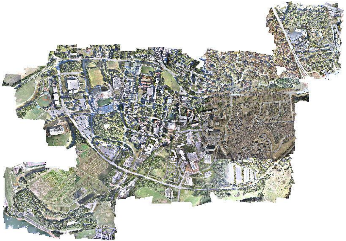
Figure 7 Completed georeference mosaic of Clemson University. This seamless orthomosaic was used for tree inventory acquisition
