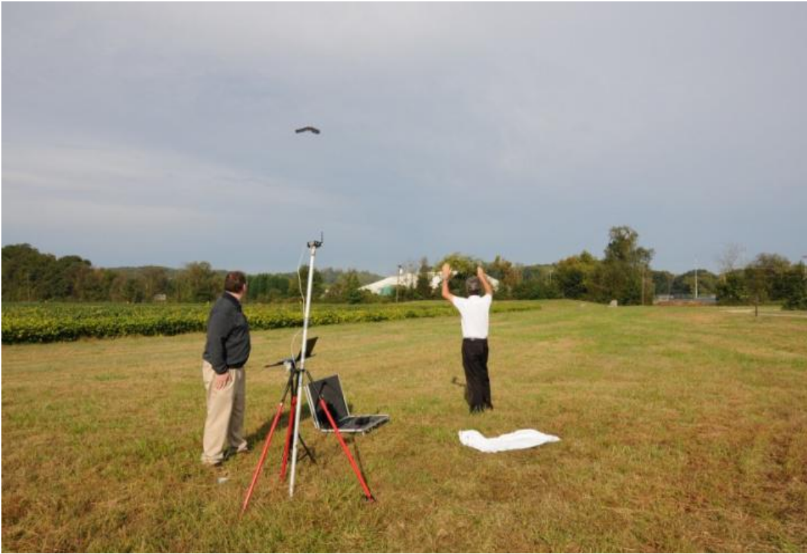
Figure 4 Ground control station for Sensefly Swinglet UAV. The control station provides continuous flight monitoring and UAV control
