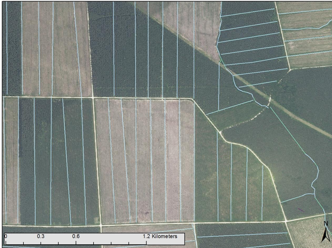
Figure 3. Linear ditch systems are maintained to regulate the water table for loblolly pine sawtimber production by Weyerhaeuser Company in the Atlantic Coastal Plain of NC. The blue linear features are the ditches and the white linear features are roads. Ditches typically border both sides of the roads in addition to inner-stand ditches. The landscape is a shifting mosaic of stand structure with dark green pine plantations and gray, young/harvested patches.
