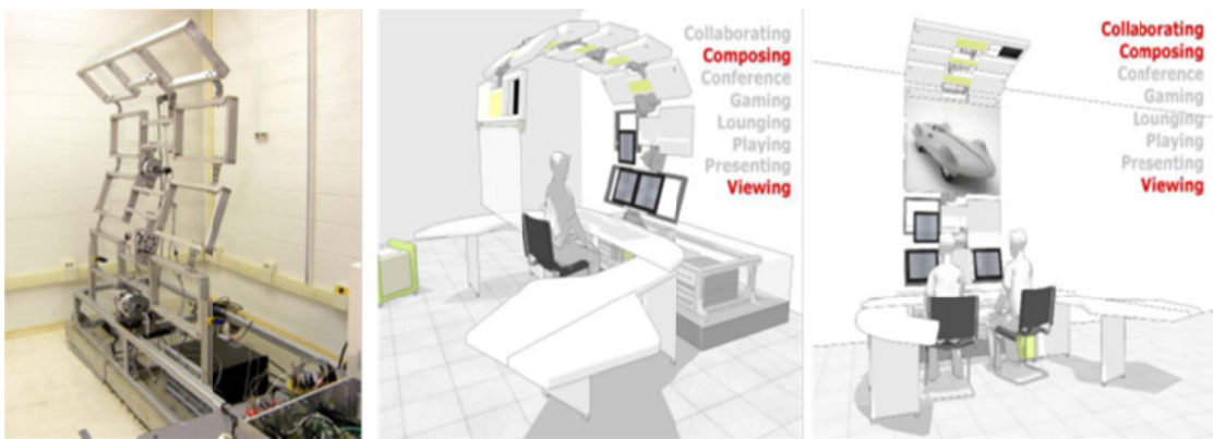
Figure 2.16 Animated Work Environment as an example for sensing physical interaction. “Developing prototype of the robotic “wall” showing four of its eight panels” (left); two different configurations for the robotic wall after physical interaction with its sensors (middle and right) (Source: Green et al., 2008)
