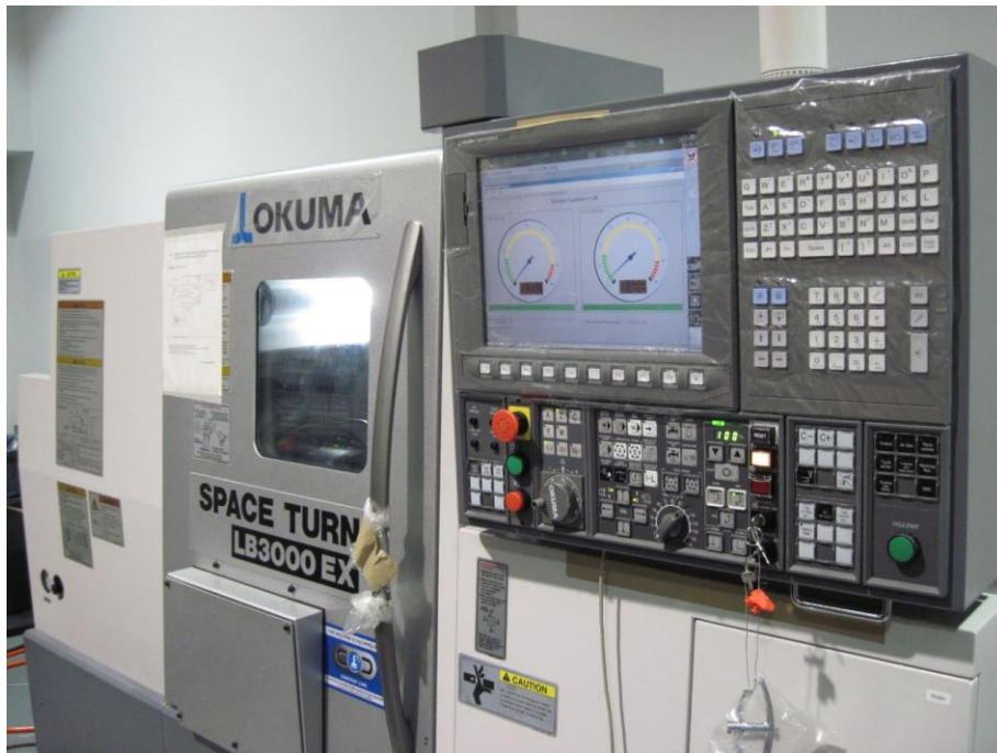
Figure 68: Software Loaded onto the Machine Control.
