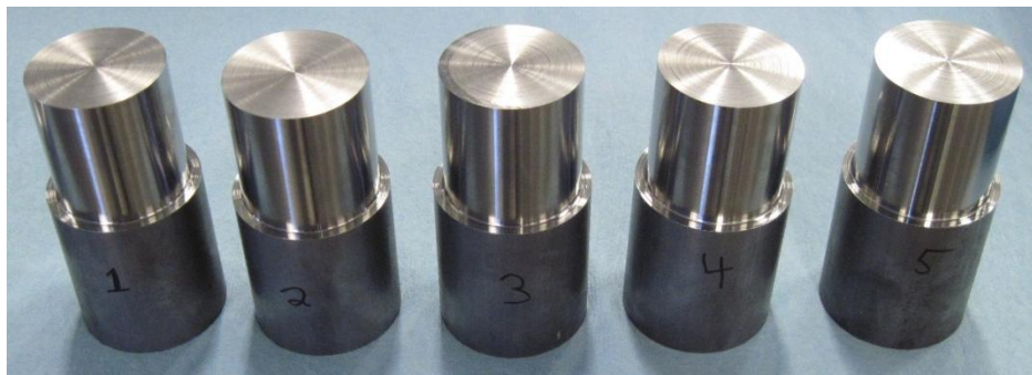
Figure J-2: Steel Specimens (Cold Roll - C-1018)
