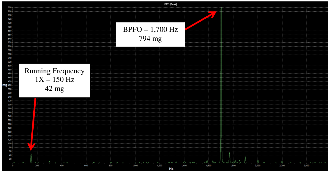
Figure 101: Frequency Spectrum at the 4.2 max dB Reading.
