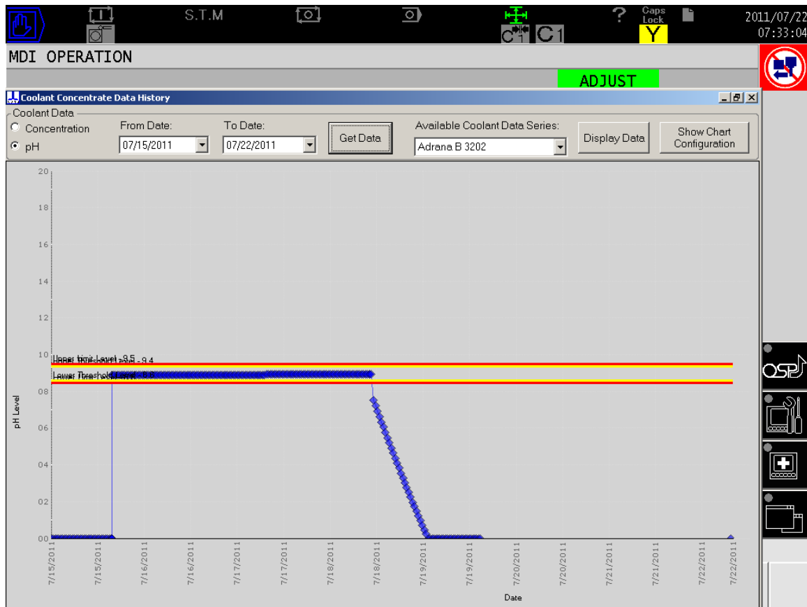
Figure 18: Okuma Coolant Monitor - History Trending.
