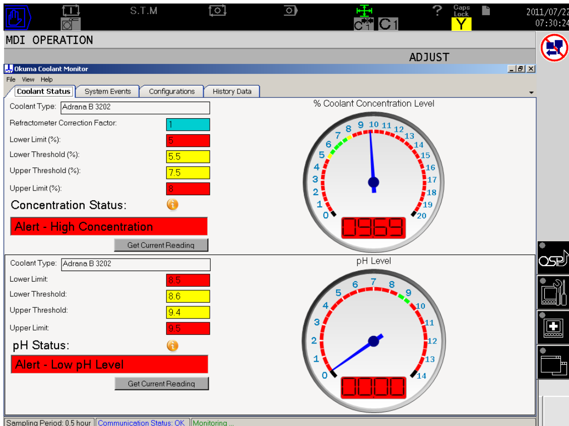
Figure 17: Okuma Coolant Monitor – Main Page.
