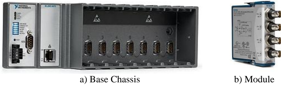
Figure 10: Example of Modular Monitoring System Hardware [27], [28].
