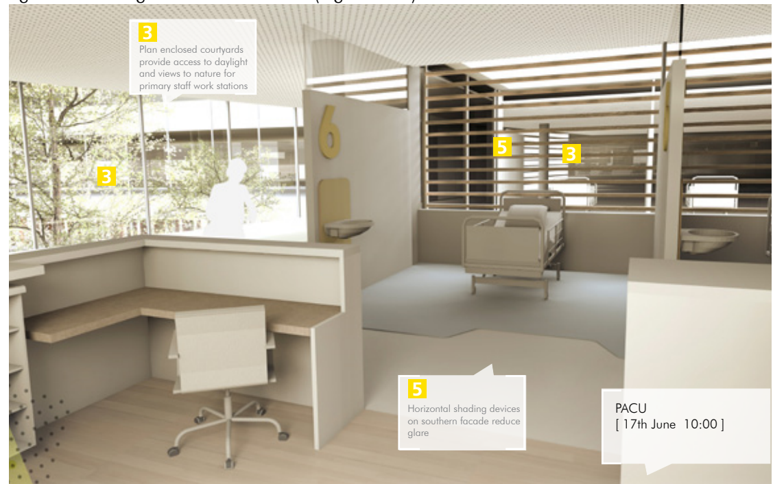
Figure 159: Primary work station in PACU with direct access to daylight and views to nature.
