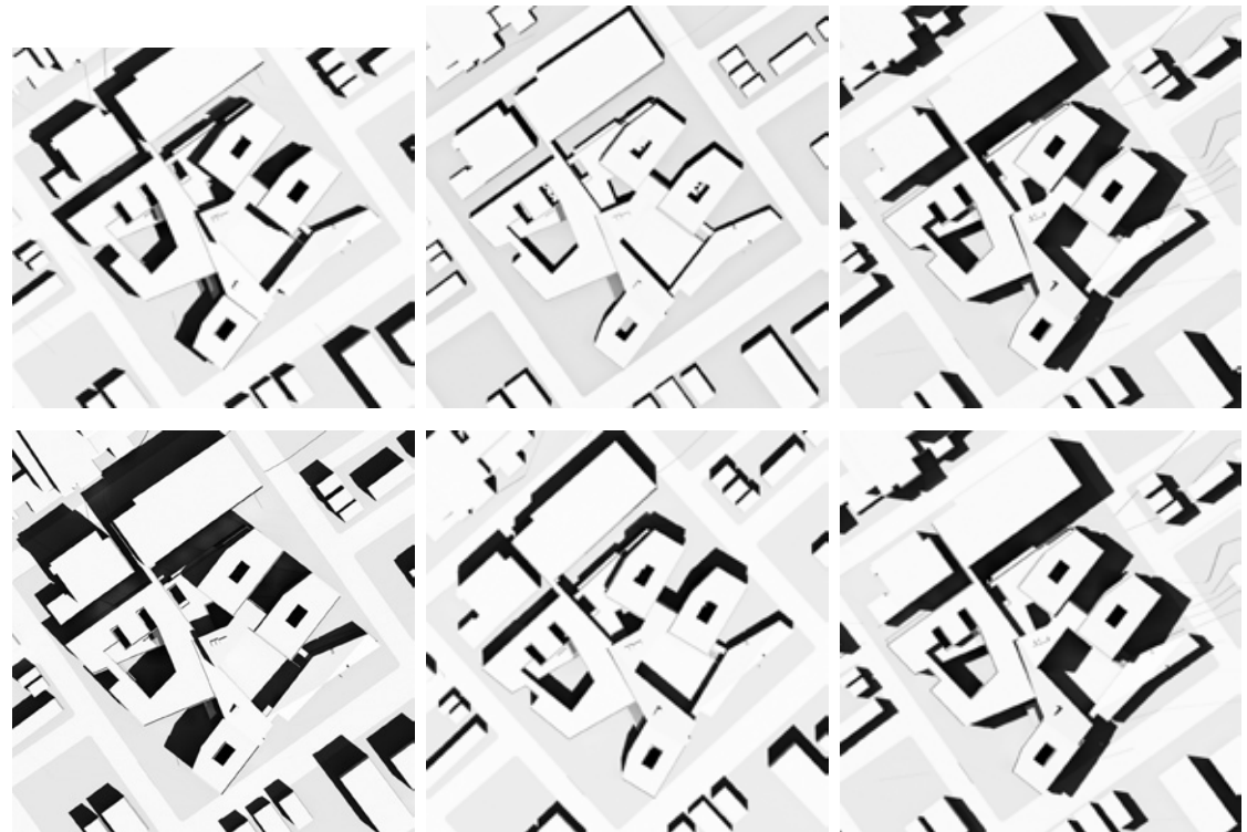
Figure 141: Daylight simulation for summer and fall/spring at 9am, 12am and 5pm
