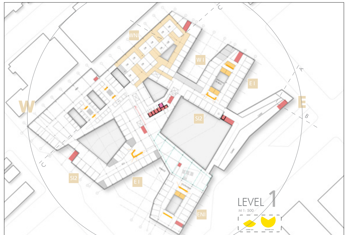
Figure 149: Floorplan level one illustrating the perforated building footprint of PACU and Surgery department (with facade matrix for shading concepts)
