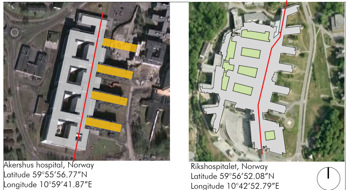
Figure 75: Hospital oriented along north/ east with inpatient units oriented east/ west.
