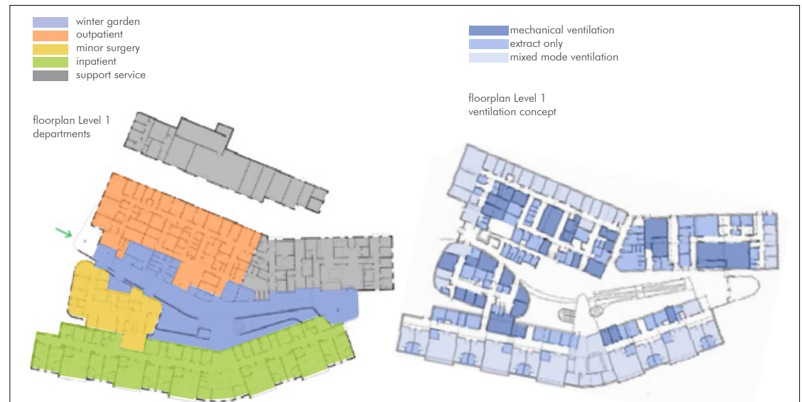
Figure 85: Department overview and ventilation concept.
