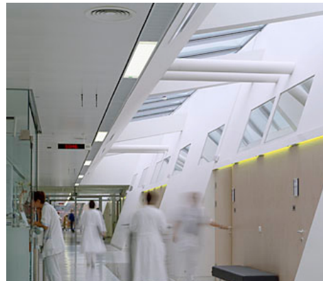
Figure 115: Deep sun penetration through skylight, mirrors and sloped walls, Knittelfeld Hospital, Austria
