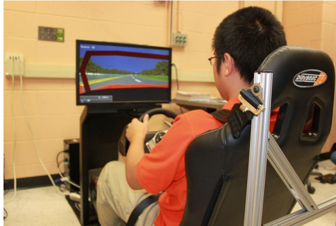
Figure 3.1: Portable Clemson Automotive Training System (CATS) with seat belt, standard human / vehicle interface, screen display, speaker and the host PC workstation
