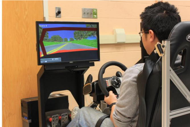
Figure 2.2: Portable Clemson Automotive Training System (CATS) with seat belt, standard human / vehicle interface, screen display, speaker and the host PC workstation
