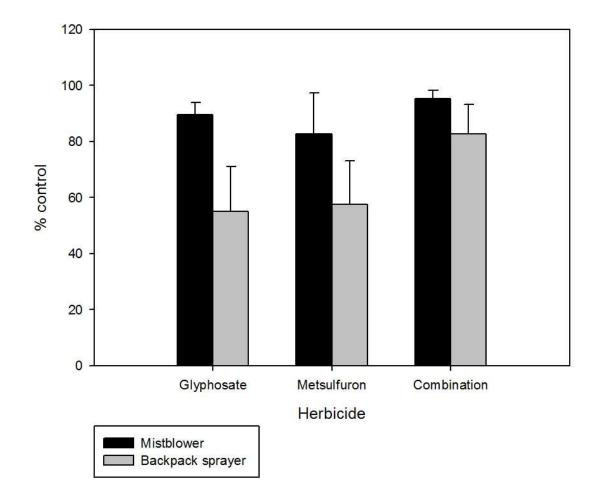
Figure 3.1. Percentage control of privet expressed as basal area by treatment (+1 SE). Mistblowers showed greater control than backpack sprayers.
