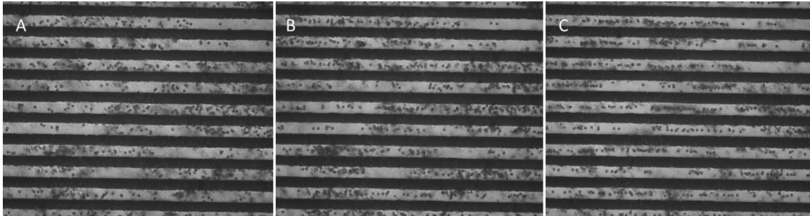
Figure 5.5: 2 \mu m beads at 314kHz, 8Vpp (A) 16Vpp (B) 24Vpp (C) in 1mM KCl
