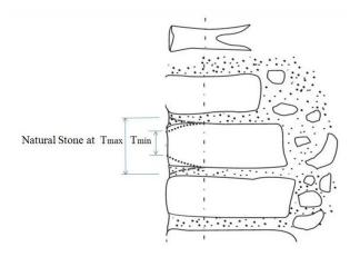
Figure 2.2. Deformation of natural stones in historical masonry as a result of thermal elongation [16].
