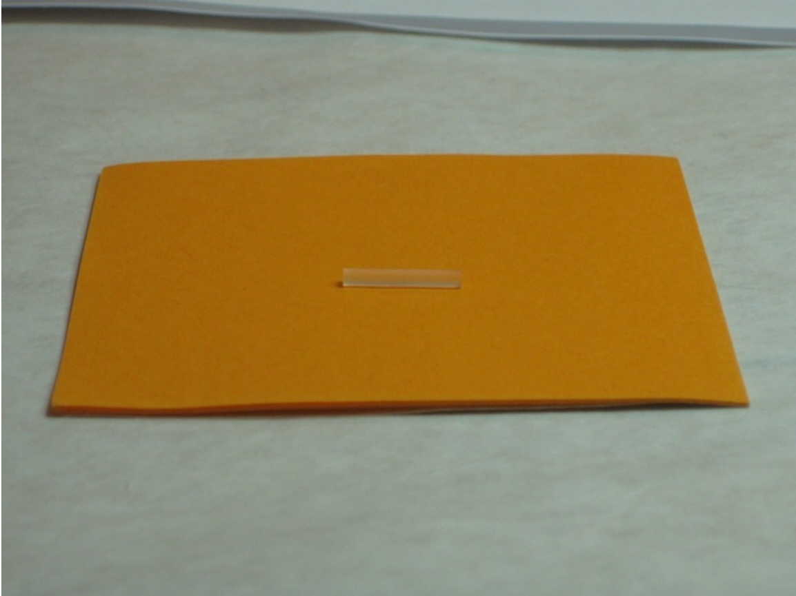
Figure 2.7: Photograph of a representative core slug drilled from the flat-index core preform.
