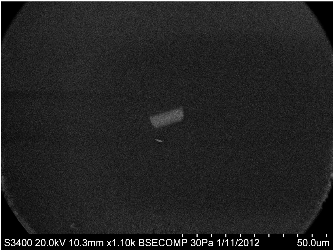
Figure 3.12: A representative SEM micrograph of the rectilinear core optical fiber.
