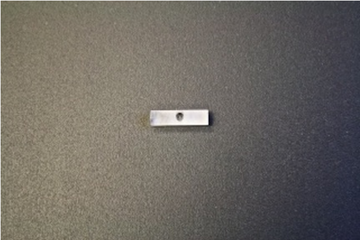
Figure 2.4: Core slug from initial preform. Note that the core does not extend across the entire diameter of the slug.
