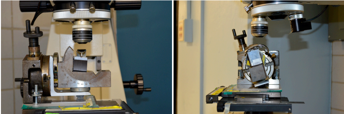
Figure 2.6: UKA femoral component mounted on customized jig and placed on stage of non-contact profilometer, demonstrating ability to control motion in frontal plane (left) and sagittal plane (right)
