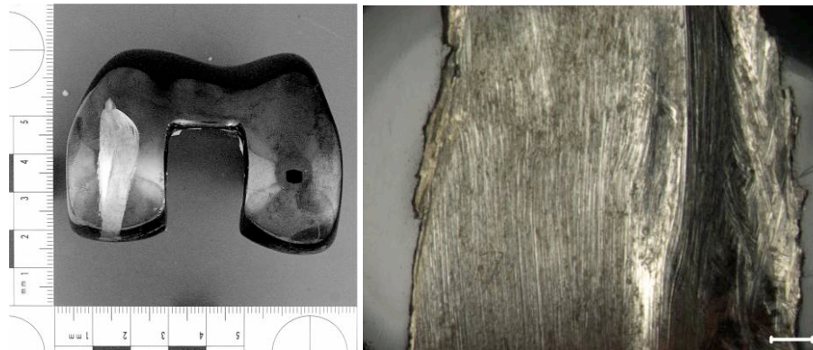
Figure 3.6: Gross image (left) and stereomicroscope image at 6x magnification (right) of gross removal of articular surface on Oxinium TKA femoral component
