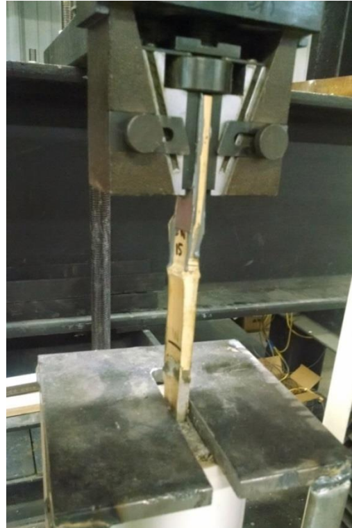
Figure 5.25 Bond specimen pullout failure
