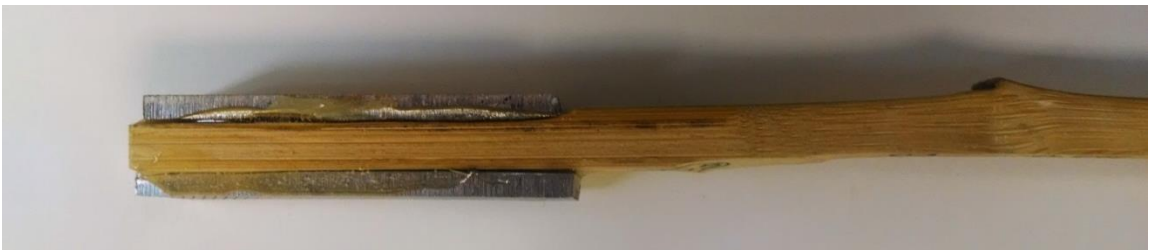
Figure 5.3 Epoxied end tab, side view
