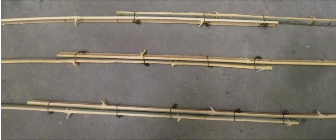
Figure 6.10 Lap-splicing of flexural reinforcement
