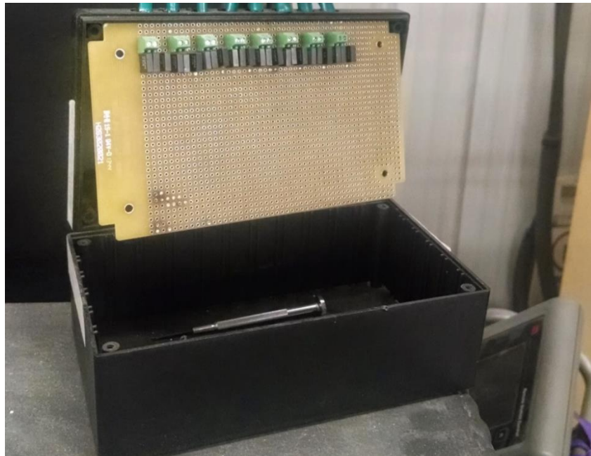
Figure 6.31 Wheatstone bridge circuit box
