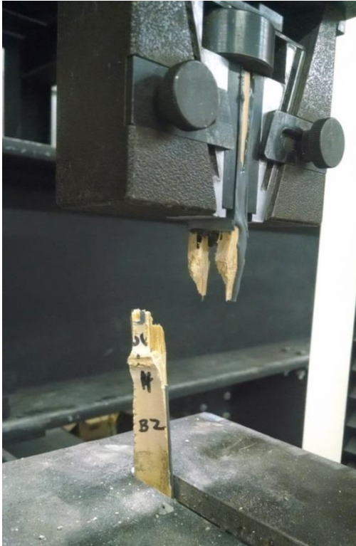
Figure 5.24 Bond specimen grip failure
