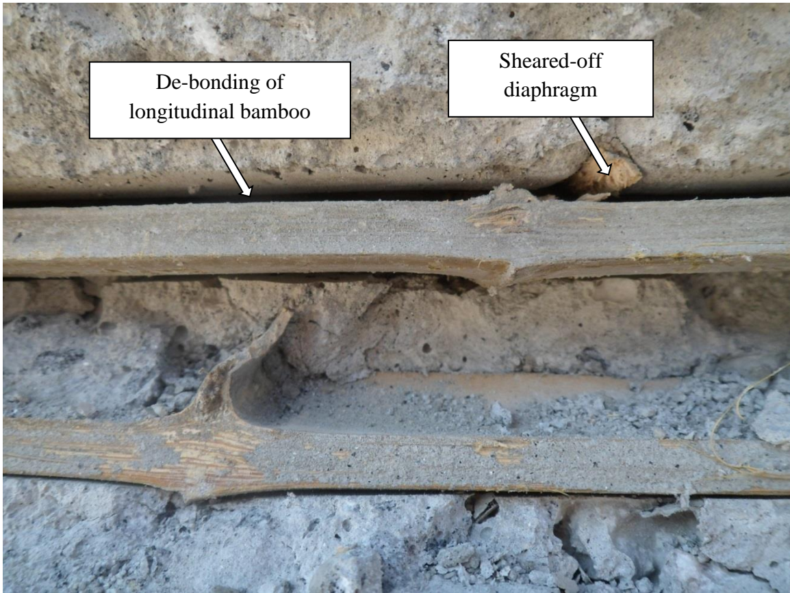
Figure 7.19 Longitudinal bamboo slippage in beam F3
