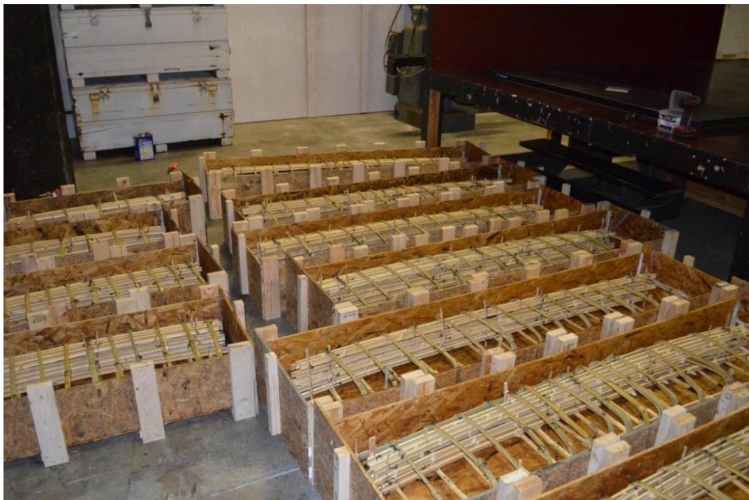
Figure 6.23 Completed forms with bamboo cages
