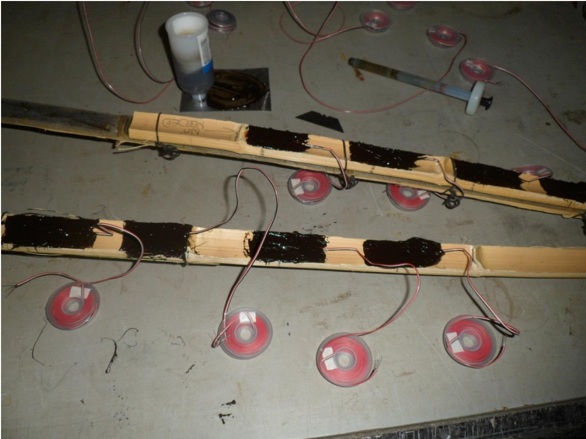
Figure 6.20 Strain gauge installation on lap-spliced reinforcement
