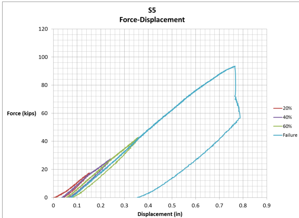
Figure 7.5 Force-displacement curve for S5
