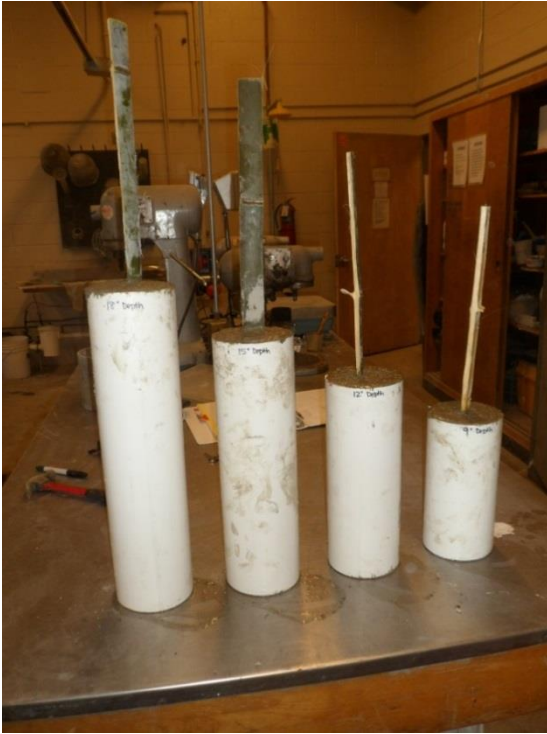
Figure 5.17 Pullout specimen embedment depths
