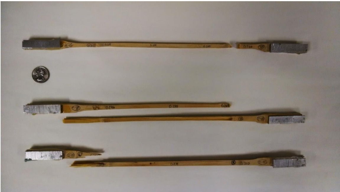
Figure 5.6 Tensile specimen failure modes
