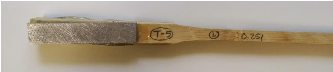
Figure 5.2 Epoxied end tab, front view
