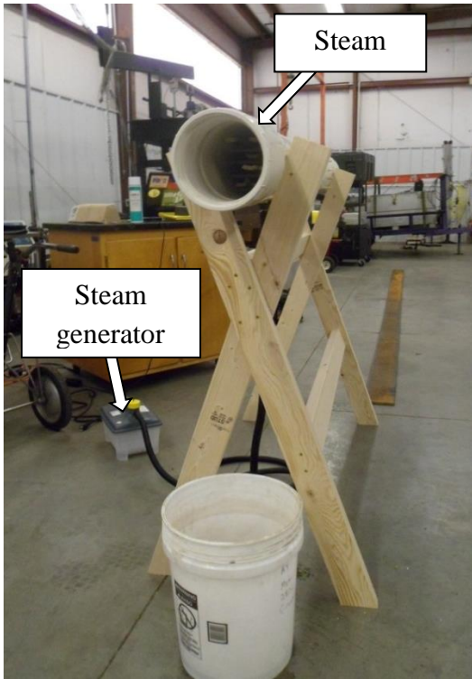
Figure 6.12 Steam box set-up
