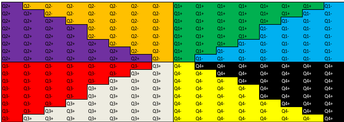
Figure 5.2: Map of the Fourier Transform of a 16 by 16 pixel window. Elements of the same color and text are individually squared, then summed, to yield an energy value for each phase angle. Bins begin with the zero to 45 degree Q1- blue section and continue counterclockwise until the final 315 to 360 degree Q4+ black section. Note that the first and final bins are adjacent to one another; this is why the circular Earth Mover's condition is valid.
