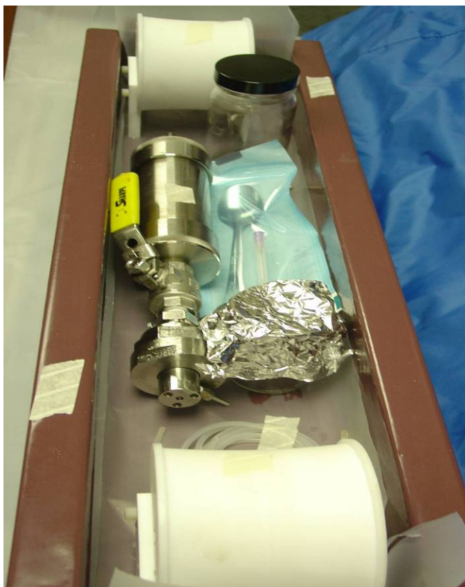
Figure 2.3: Preparation for the sterilization of the equipment items. Equipment items used in the alginate fiber spinning process were cleaned with LYSOL® All Purpose Cleaner, dried, sprayed with 70% ethanol, and placed inside a pre-cleaned basin.
