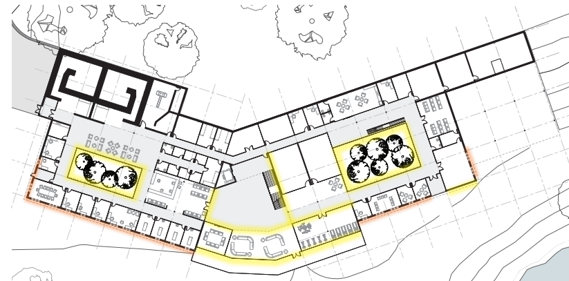
Figure 115: provision of daylight on the lower floor
