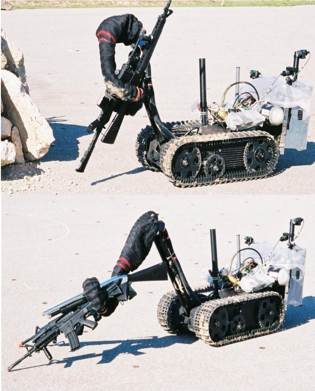
Figure 2.9 OctArm grabs and then drags away multiple air-soft guns.
