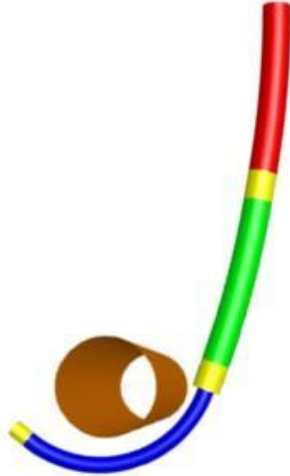
Figure 4.2 Illustration of a manipulator in a local minimum configuration.
