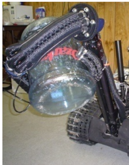
Figure 2.1 OctArm V grasps a water jug, guided by the user interface.
