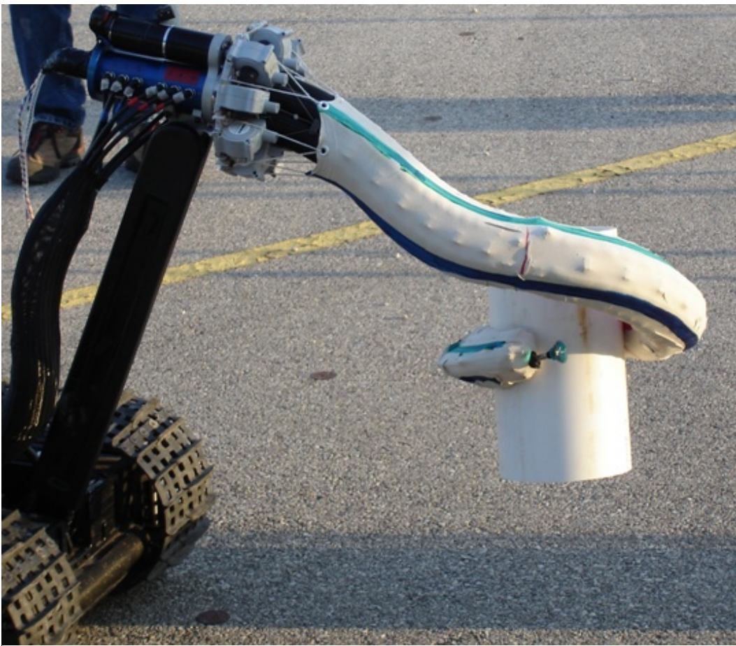
Figure 2.8 OctArm holds a PVC pipe with the aid of a high-friction, latex skin.
