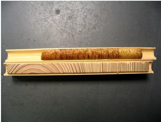
Figure 9: Historic Deerfield's Architectural Conservator, Bill Flynt's, Pitch Pine Cores: Before and After Sanding
