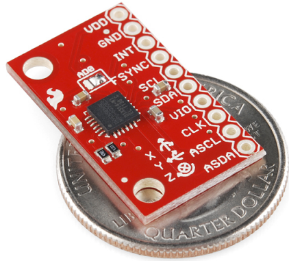
Figure 2.5: A breakout board containing the MPU 6050 chip. Quarter shown for comparison.
