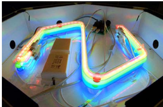
113. Digital Sensors Integrated into Lighted Floor Panel - ADA 2001 // Architectural Design
