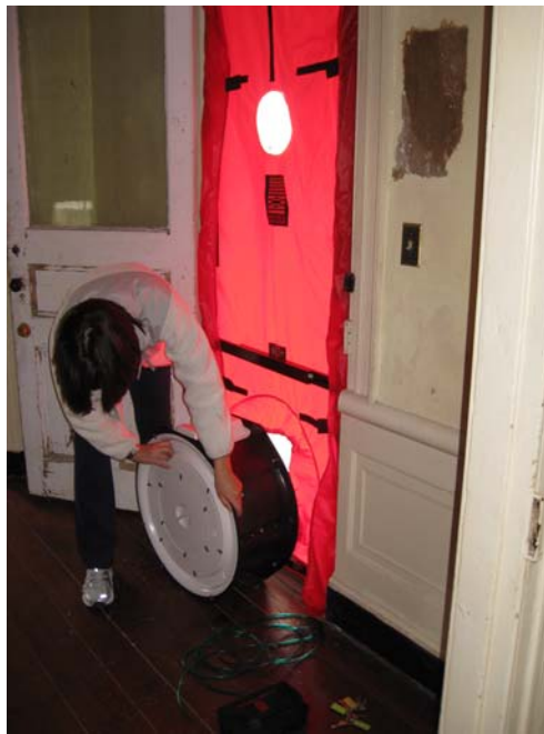
Figure 3: Blower door setup at 63 Smith Street. Photo courtesy April Wood.
