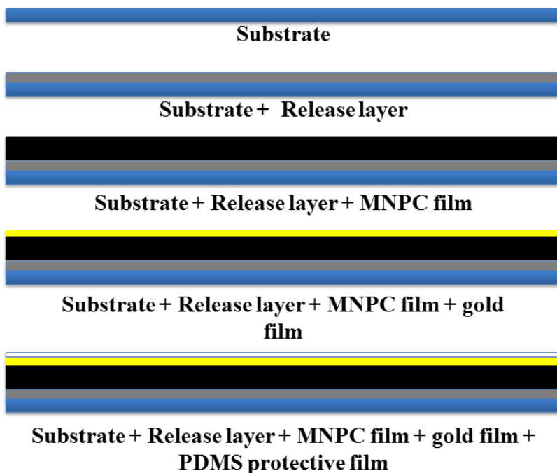
Figure 3.1: This depiction shows how the layers of the film system will result after the MNPC construction process is completed. It should be noted that only the gold and MNPC layers will be used for bulge testing and magnetic deflection testing.
