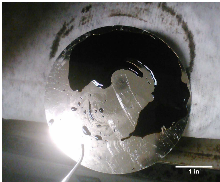
Figure 4.14: MNPC film sample that did not crosslink after deposition, evident by the visual appearance of the mirrored steel substrate.
