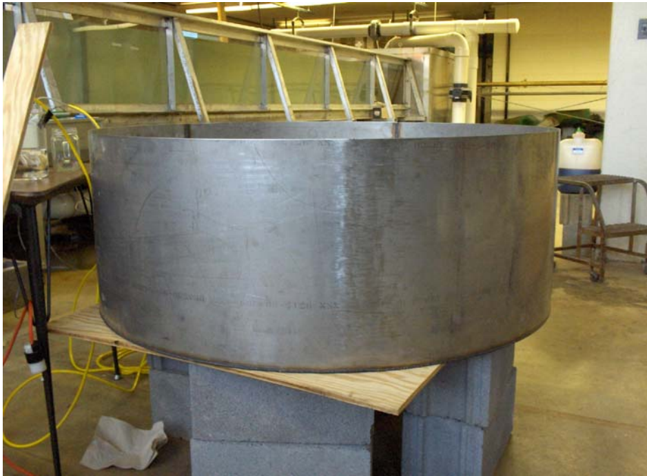
Figure 3.1: Stainless Steel Pan (4-ft diameter and 18-inch depth)
