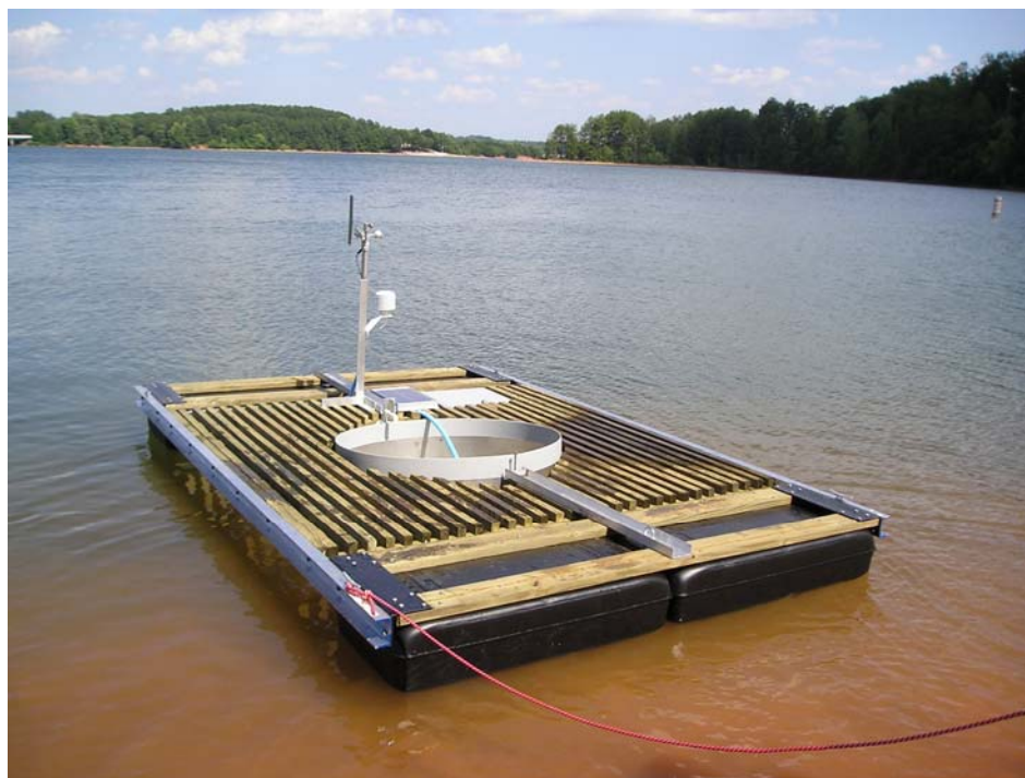
Figure 3.18: Floating Evaporation Pan Complete Setup on Lake Hartwell
