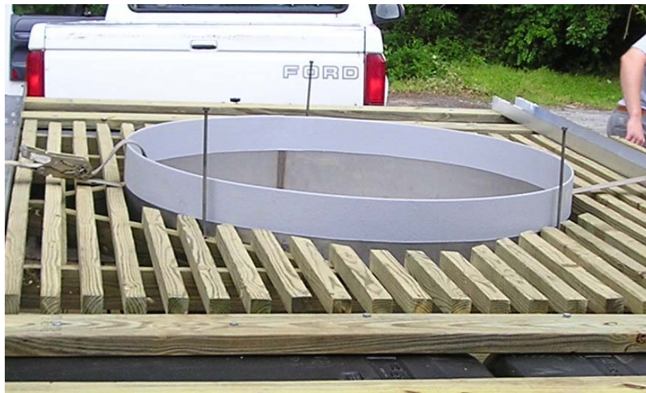
Figure 3.8: Metal Rods Connected to Pan and Wooden Frame
