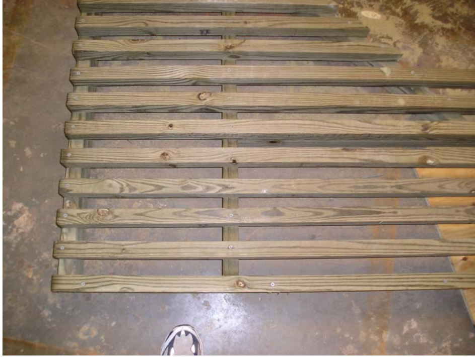
Figure 3.6: 8-ft x 8-ft Wooden Frame (spacing of wooden boards)
