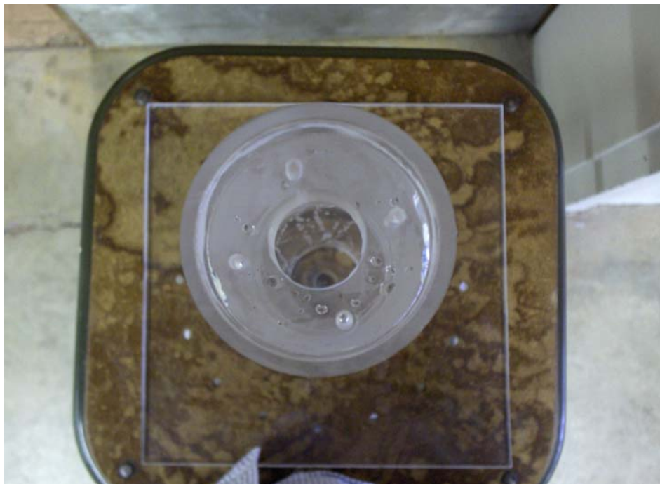
Figure 3.11: Plexiglas Cylinder Four 1/16 th -inch Holes (top view)
