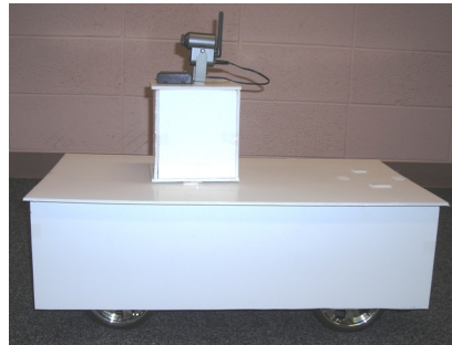
Figures 6a and 6b: Camera placement at the rear of the robot for the in view condition (6a) and camera placement at the front of the robot for the not in view condition (6b).
