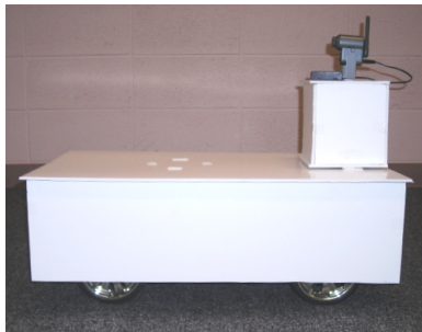
Figures 6a and 6b: Camera placement at the rear of the robot for the in view condition (6a) and camera placement at the front of the robot for the not in view condition (6b).
