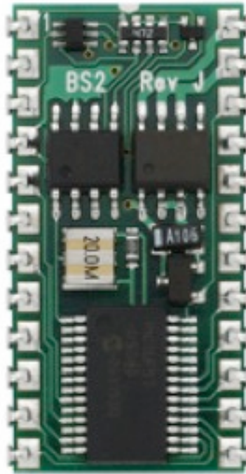
Figure 16. Basic Stamp2® microcontroller (Parallax, 2008)
