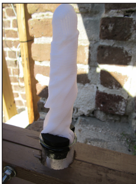
Figure 3.12: Test tube wrapped in gauze to collect airborne soluble salts (photo by author)
