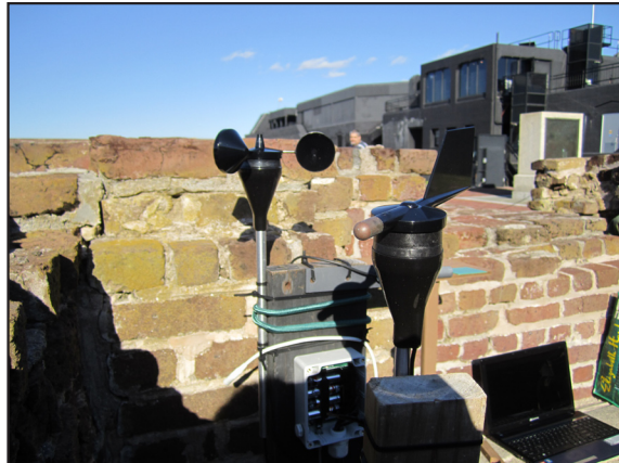
Figure 3.7: Anemometers in place at Fort Sumter National Monument (photo by author)
