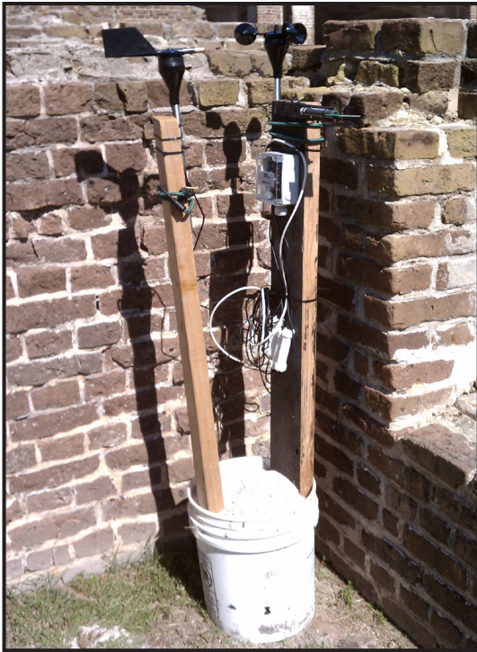
Figure 3.3: The datalogger was secured in a bucket of sand to prevent having to anchor the system to the historic masonry (photo by author).
