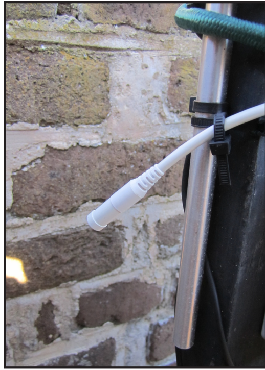
Figure 3.4: Onset temperature/RH sensor (photo by author)
