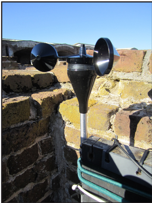
Figure 3.5: Onset wind speed sensor (photo by author)
