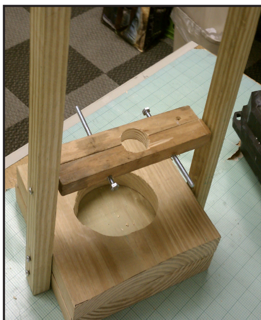
Figure 3.11: Bolt assembly to secure flask to weather shield (photo by author)
