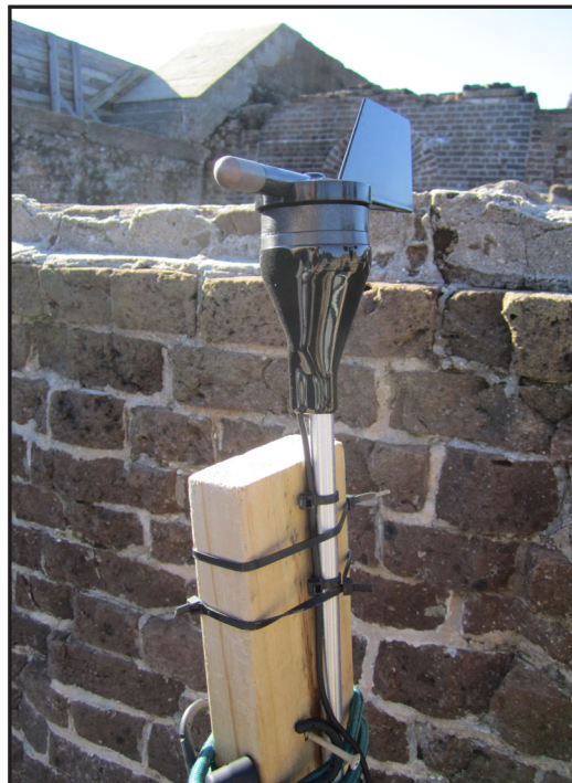
Figure 3.6: Onset wind direction sensor (photo by author)
