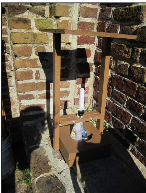
Figure 3.9: Airborne chloride test in place at Fort Sumter. (photo by author)
