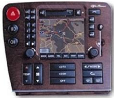
Figure 6 VW Beetle interior parts, Central console cockpit on the Alfa 166 in Bayblend®
