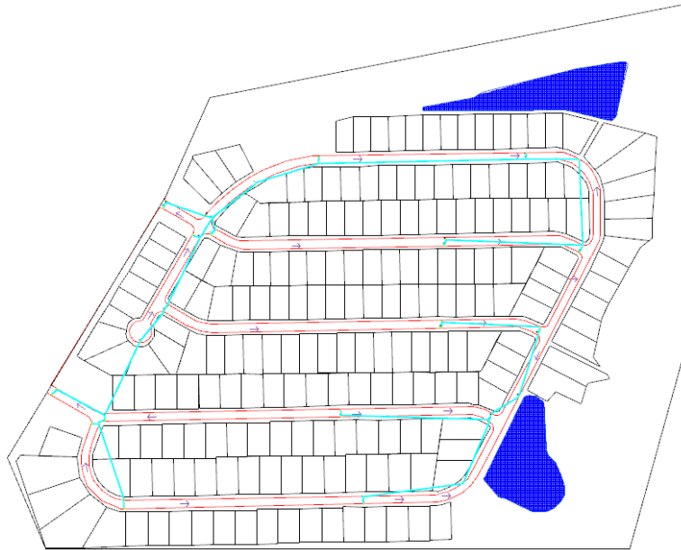
Figure 3-3 Residential site layout with 178 lots and two detention ponds. Storm sewer piping is shown in blue and connects at each stormwater inlet. Due to topography of site, two ponds exist.
