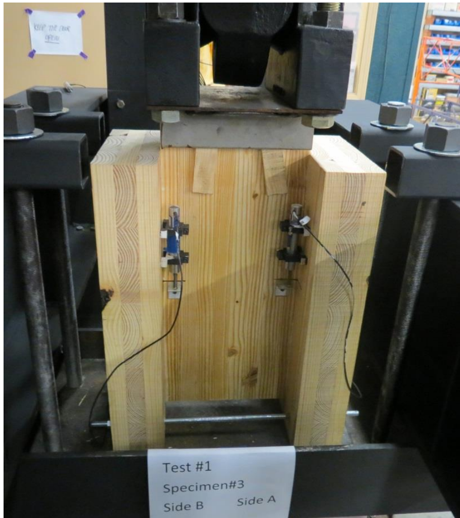
Figure 4.11: Test Specimen Reinforced with Rods
