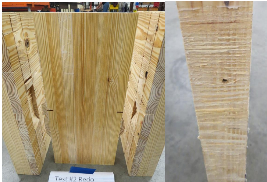
Figure 4.46: Examples of Shallow and Deep Rolling Shear Failure Modes
