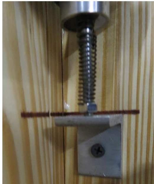
Figure 4.9: Set Up of LVDT Sensors
