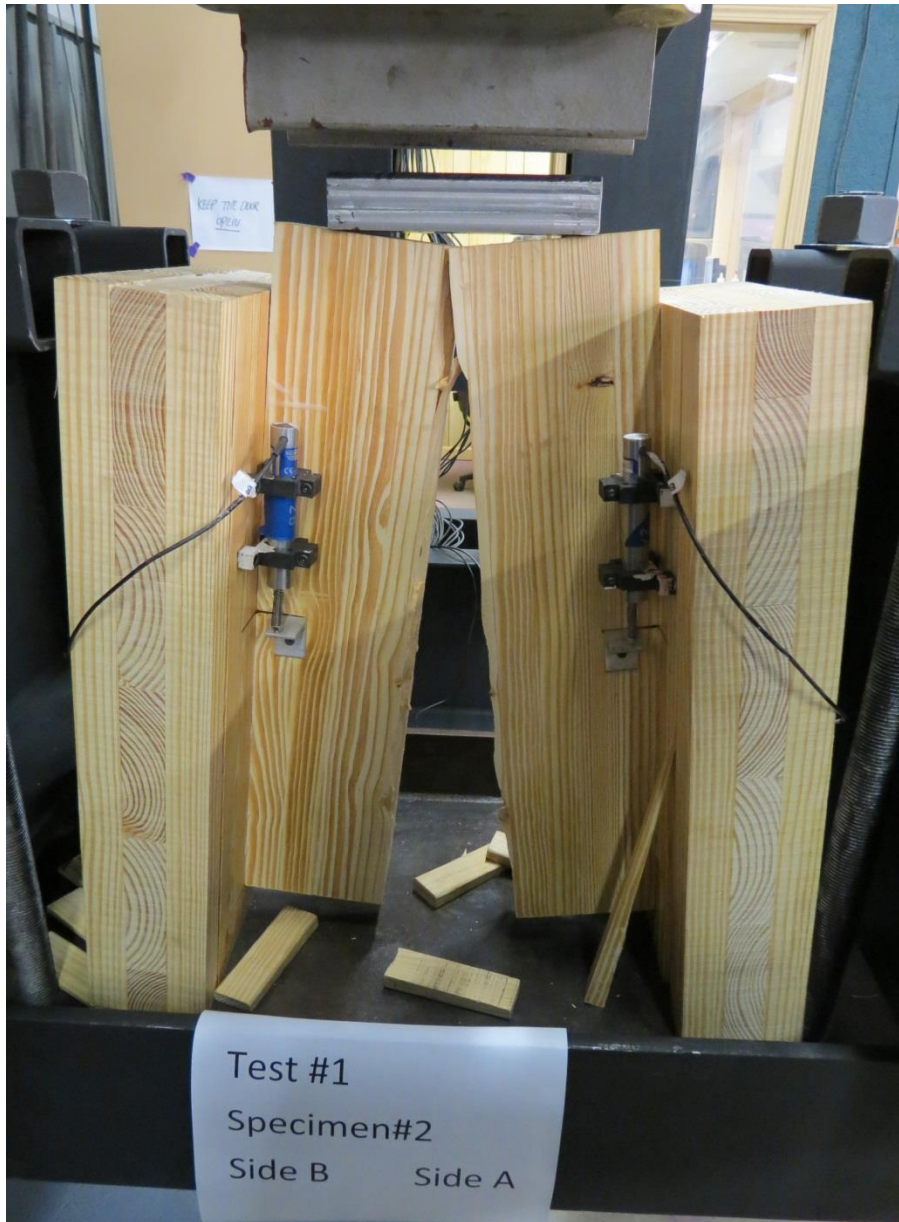
Figure 4.10: Bending Perpendicular to the Grain Failure Mode
