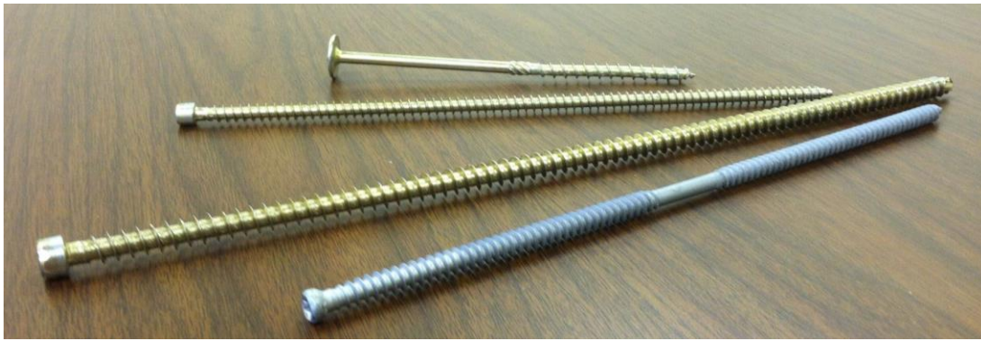
Figure 4.18: ASSY and SFS Intec Screws Used for Testing
