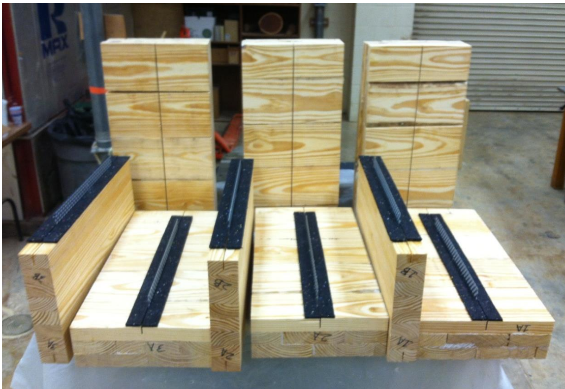
Figure 4.37: Gluing Together HBV Specimens
