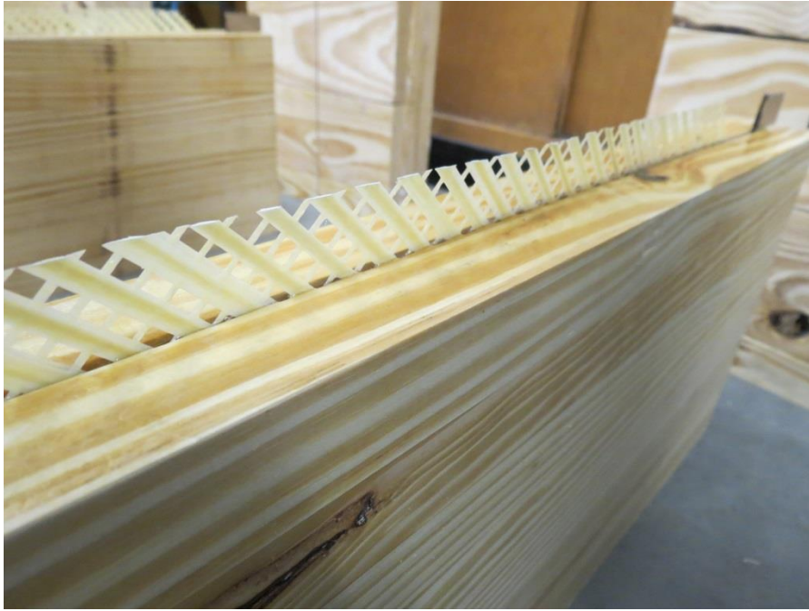
Figure 4.39: Test #16 – Embedding GFRP Fabric
