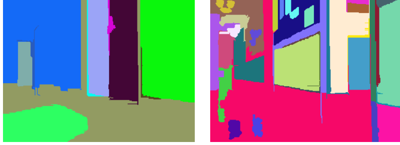
Figure 2.8: The result of graph-based segmentation [11] on two corridor images used in Figure 2.7, with each region assigned a random color. Note that the floor is almost a homogeneous area in both images, while the wall and doors are divided into several smaller regions.
