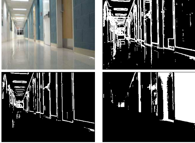
Figure 2.3: TOP-LEFT: A typical corridor image. TOP-RIGHT: Pixels with gradient magnitude greater than a threshold are shown in white. BOTTOM-LEFT: Using the separating curve from Figure. 2.4, the edge pixels mostly follow the boundaries of the wall, door frames, and floor. BOTTOM-RIGHT: The original image thresholded by a value determined by the separating curve, thus revealing the structure of the corridor.
