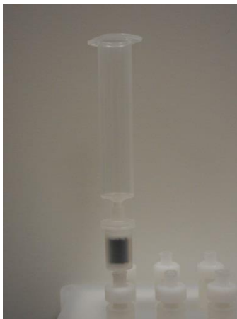
Figure C.1 Reservoir, cartridge, vacuum manifold set-up
