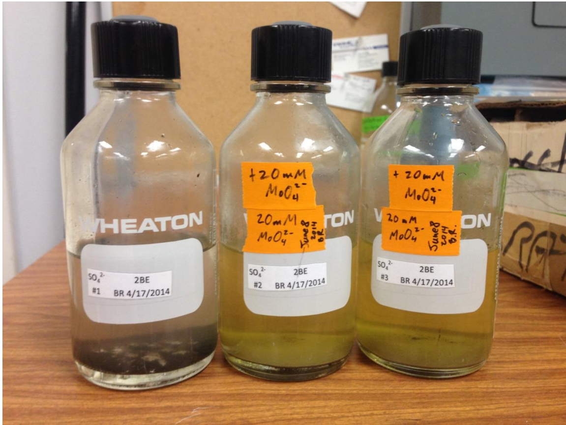
Figure J.2 Photograph showing the unamended first transfer enrichments on day 67. Bottle #1 is on the far left; it contains no molybdate. Bottles #2 & #3 are center and far right, respectively; bottles #2 & #3 contain 40 mM molybdate.
