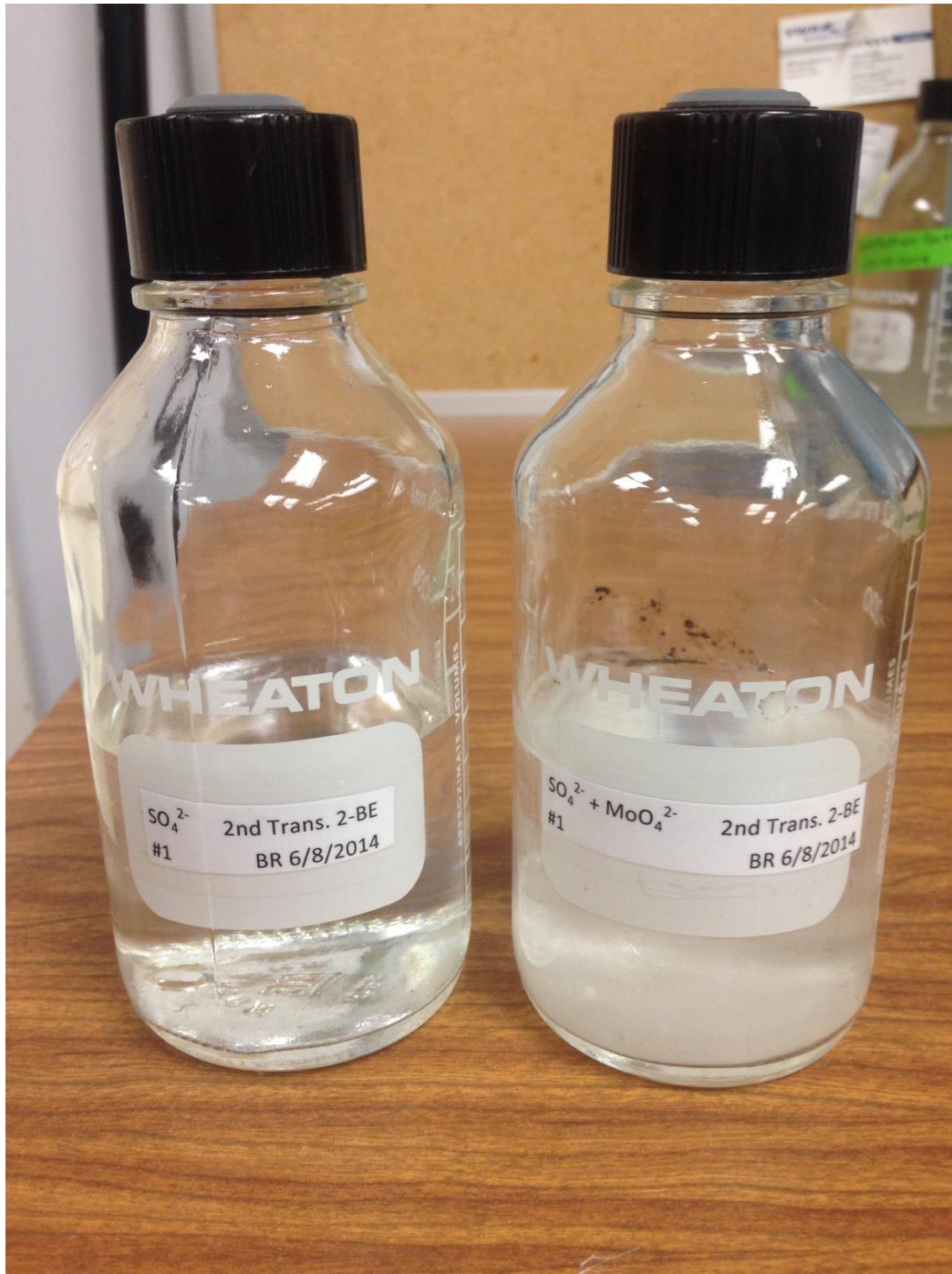
Figure J.3 Photograph showing the precipitate which formed a hazy crust on the glass surface in the 20 mM molybdate spiked second transfer enrichment (left), and the clear unamended second transfer enrichment (right) on day 17.
