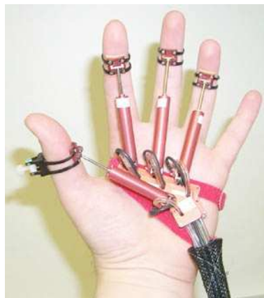
Figure 3: Haptic grasper developed at Rutgers University.
