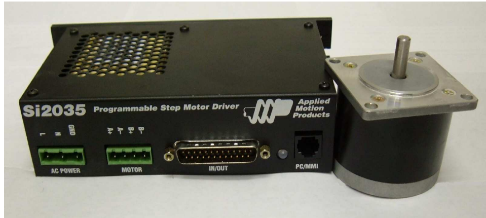
Figure 2.2: An external view of the Applied Motion 2035i stepper motor driver and stepper motor.
